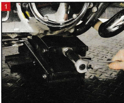
Use a center jack to support the frame of the motorcycle.
