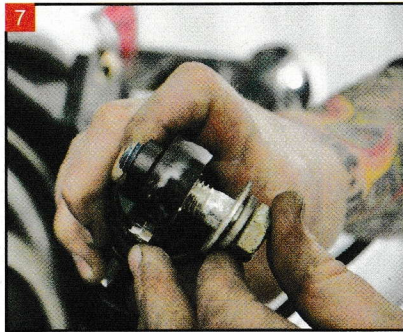
7 Use the stock shock bolts with the new Super Shox and included spacers.
