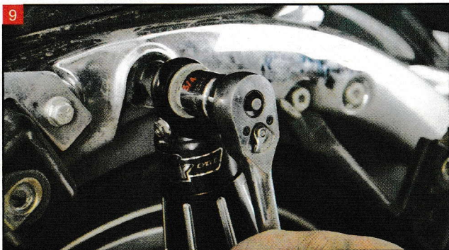
9 Using a 3/4" socket, begin to tighten down both shock bolts.
