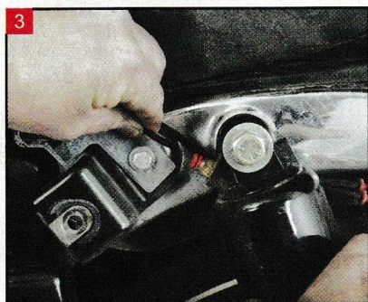
Disconnect the air lines from the stock shocks.
