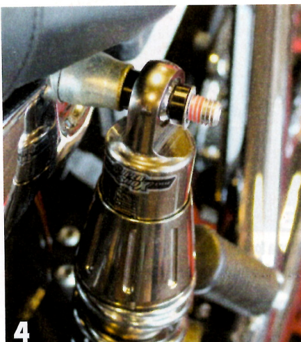
4 Install the new Super Shox top mount with a supplied black spacer on either side of the bracket and a washer on the stock washer on the outside.
