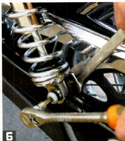
6 Install the new Super Shox bottom mounts with a supplied black spacer on either side of the bracket. Use a T50 Torx on the right side and torque to 30-40 ft-lbs.; use a 3/4" wrench and a T50 Torx on the left side.
