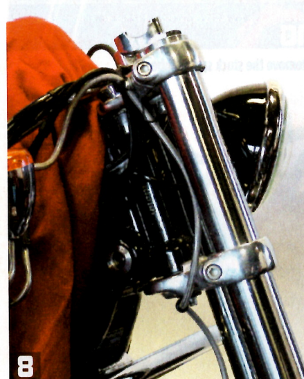
8 Now on to the front suspension. Ron already has his handlebar clamp removed and the handlebar sitting on the covered gas tank.
