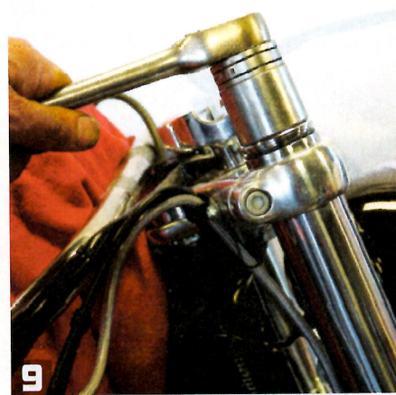
9 Using a 1-3/8" socket, remove the fork cap. Be careful as the spring is under pressure and will pop up. Press down as you twist to keep it in place.
