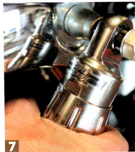
7 Adjust preload based on the supplied scale from Super Shox. Ron's setting it at level 1. When his daughter, Olivia, hops on, he'll readjust as necessary.
